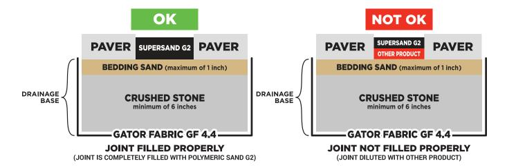
NEVER USE SUPERSAND G2 WHEN PAVERS ARE INSTALLED ON A CONCRETE SLAB. INSTEAD, USE ALLIANCE GATOR MAXX G2.
